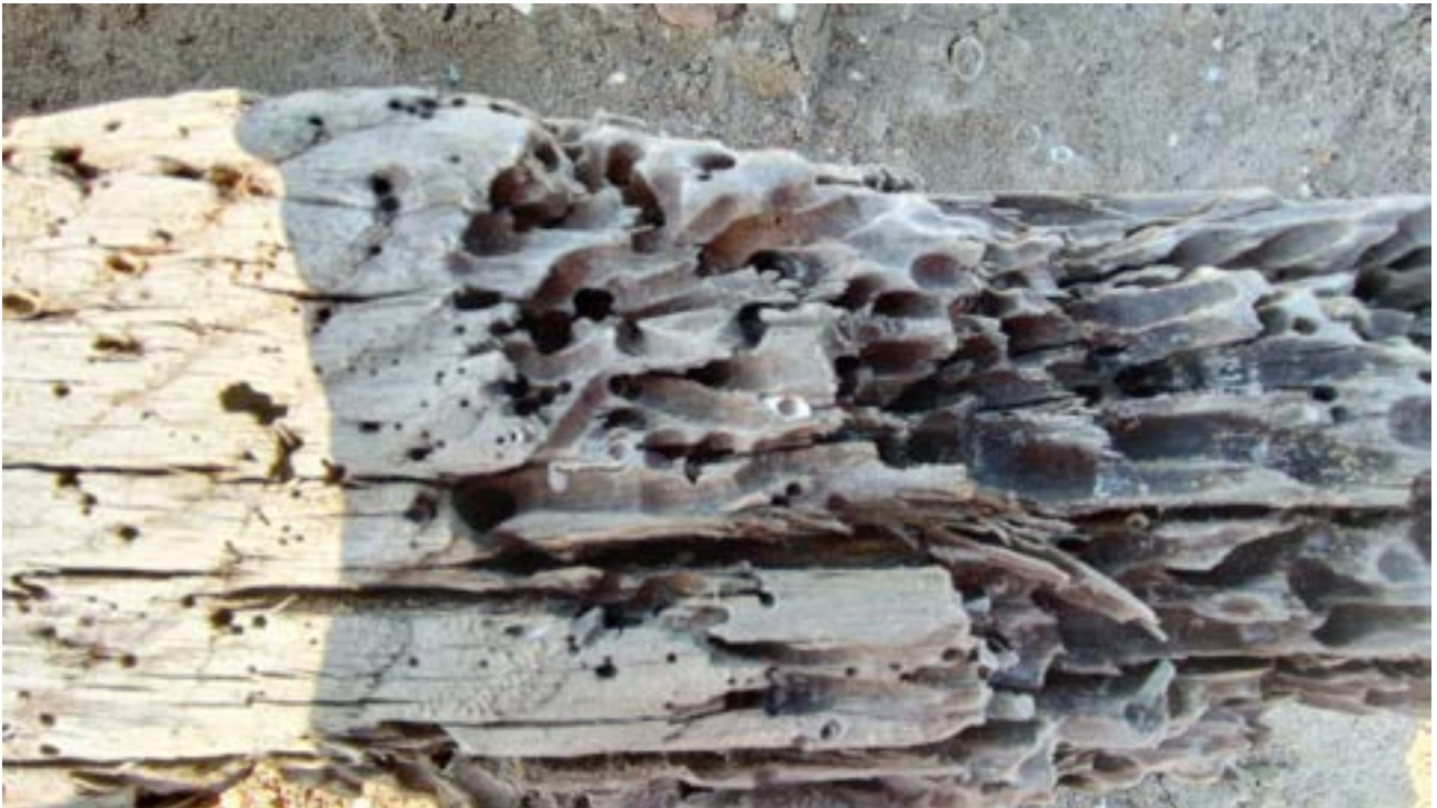
An Ottoman ship timber affected by Teredo Family (Photo Metehan Samet Gül)
